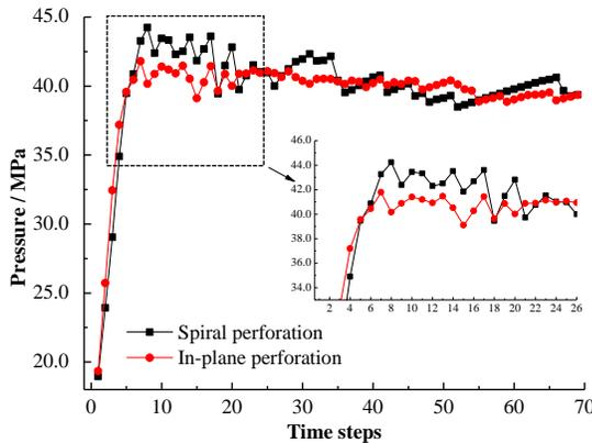
Fig. 9 Comparison of pressure change with different perforation strategy
