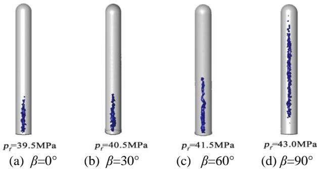
Fig. 6 Initial fracture geometry for different perforation deflection angle  $\beta$
