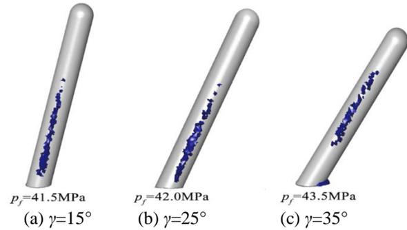
Fig. 7 Initial fracture geometry for different perforation incline angle  $\gamma$
