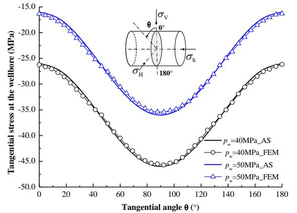
Fig. 4 Tangential stress distribution along the open-hole horizontal wellbore
