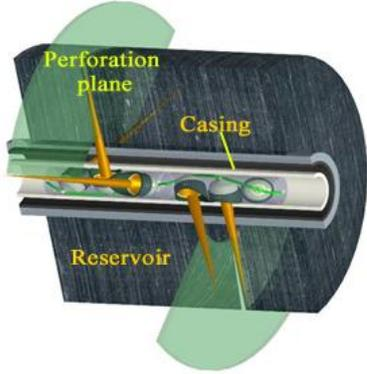
Fig. 1. Schematic diagram of in-plane perforation (Liu et al. 2014)
