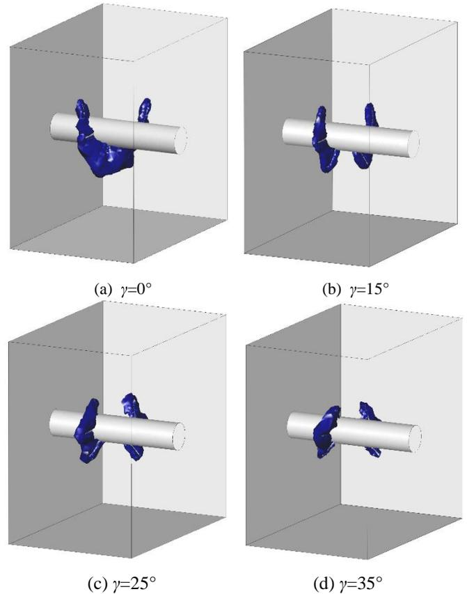
Fig. 10 Fracture geometry of near-wellbore for different incline angle  $\gamma$
