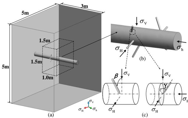
Fig.3 Computational geometry models (a) Model geometry; (b) In-plane perforation model; (c) In-plane perforation angle parameters.
